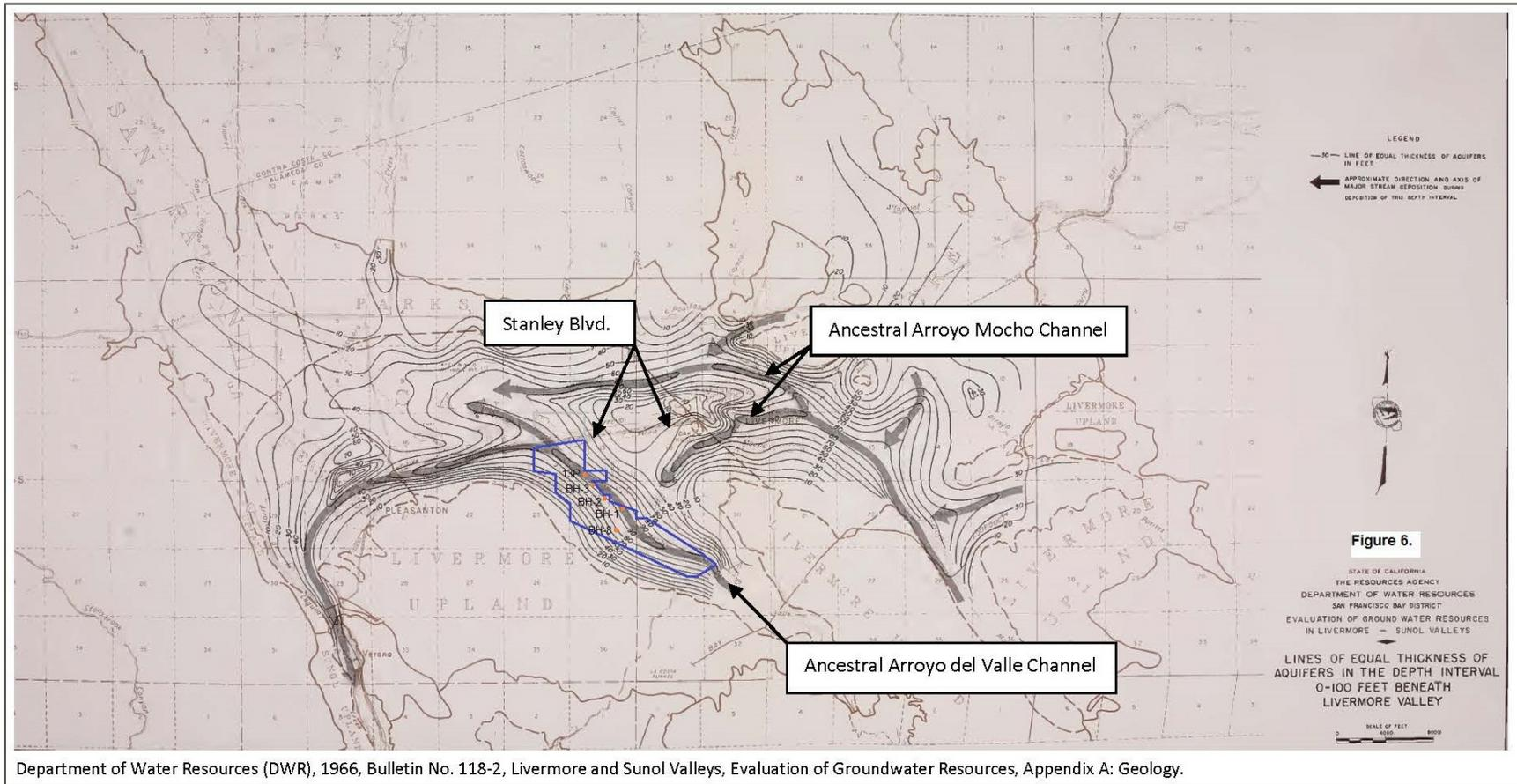
**Lines of Equal Thickness of Aquifers in the Depth Interval 0-100 Feet**
